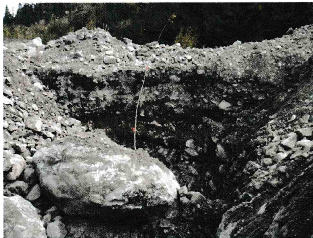
Plate 6: Very large boulder encountered in H1
