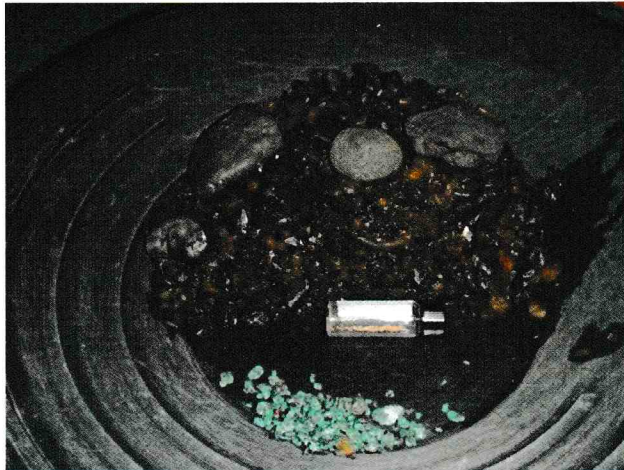
Plate 4: Magnetite, copper and gold recovered from sample H4 10-15'
